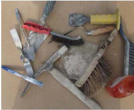
Lime mortar tools. These are the main tools you will need for pointing stone and brick and filling in cracks and gaps using a lime mortar. See pointing picture on the last page of this article.
